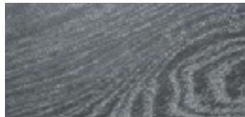
ER (registered emboss): genuine wood appearance due to consistence between pattern and embossing
